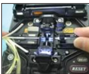
2. Slide splice sleeve over splice point.
