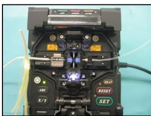
1. Set cable and connector plug on fusion splicer and splice.
